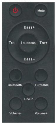
red button turns the unit on or back into standby
