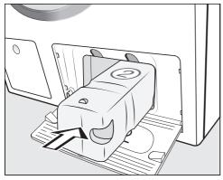
Push the UltraPhase 2 detergent cartridges into compartment 2 until it locks into position.
