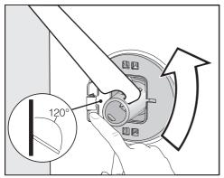
Open the cover and use the wrench supplied with the washing machine to turn the shipping strut 90°.
