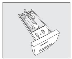
Remove the insert. Clean the insert thoroughly with warm water.
