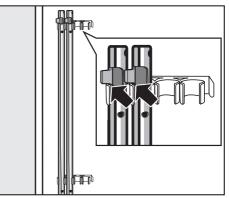
Secure the shipping struts to the back of the washing machine. Make sure that the top catch is located above the holder.
