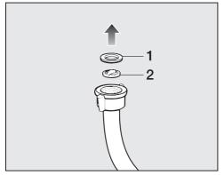
Remove the rubber seal 1 from the connector.
