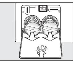
Remove the drain filters completely.
