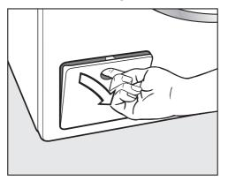
Open the drain pump flap.
