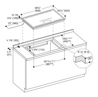
Minimum countertop thickness ¾" (20 mm) for surface mounted installation.
