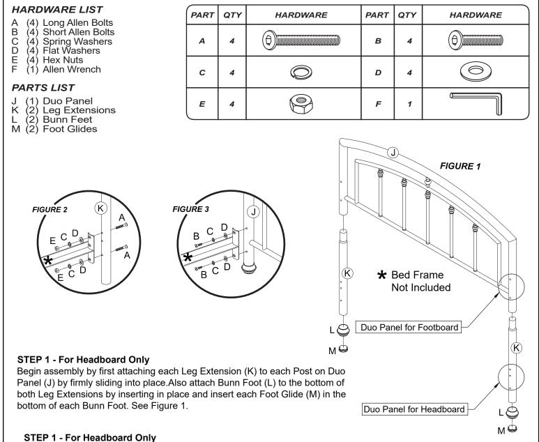
Begin assembly by first attaching each Leg Extension (K) to each Post on Duo Panel (J) by firmly sliding into place. See Figure 1.
