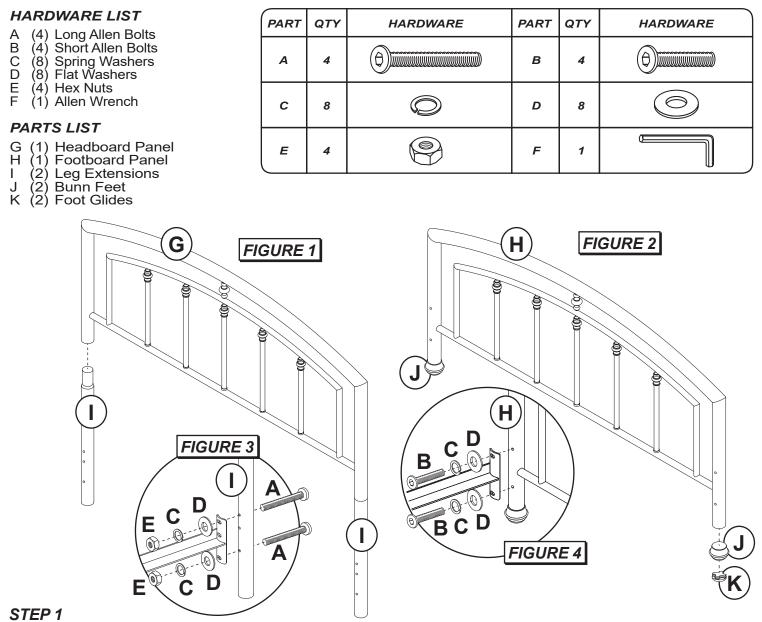
Begin assembly by first attaching Bunn Feet (J) to bottom of posts on Footboard Panel (H). Next attach Foot Glides (K) into Bunn Feet (J). See Figures 1 and 2.
