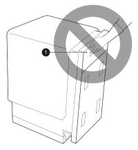
• Do not push the door of the dishwasher with knees when sliding the dishwasher into position. Doing so can damage the front cover.
