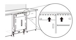
2 Measure the difference in height (x") between the top of the dishwasher door and the tops of the surrounding cabinet doors or drawers.
