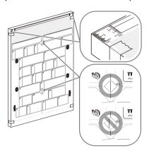
3 Use a 1/16" (2 mm) diameter drill bit to drill 3/8" (10 mm) deep pilot holes at the 12 points marked on the template.
