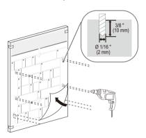
Remove the template, and attach the upper and middle panel brackets (provided) to the cabinet panel using the provided wood screws.
