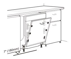
2 Attach the cabinet panel to the dishwasher door on the sides using the provided bracket screws.
