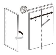
Align the top and center line on the installation template with the top and center line of the cabinet panel. Securely tape the installation template to the back of the cabinet panel.
