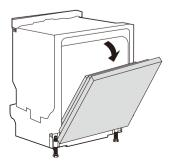
2 Use the door adjustment screws provided to adjust the door spring tension at the bottom of the dishwasher.
