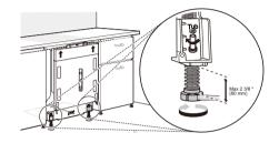
If a flat-blade screwdriver is unavailable, use a 1/4" square drive wrench(1) or 3/8" square drive wrench(2) with 1/2" socket(3) to turn the front leveling feet and adjust the front of the tub.
