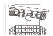
There is a 24 \% inches (56 mm) gain in height when the upper rack is moved to the lower position.
