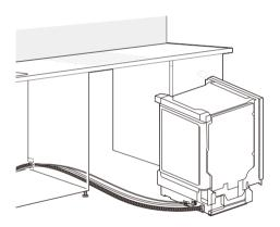
2 Smooth out or pad the edges of the hole drilled for the water supply to avoid damaging the drain hose.
