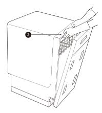
Align the dishwasher with the opening. Make sure the water supply line and power cord extend smoothly without kinks or bends.
