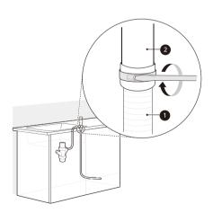
If it is not connected, attach the rubber hose connector to the disposal or waste tee with a hose clamp (not provided).
