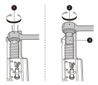
Adjust the front and rear leveling legs until they are all in firm contact with the floor. Failure to level the dishwasher may prevent the door from closing properly and the dishwasher will not turn on.
