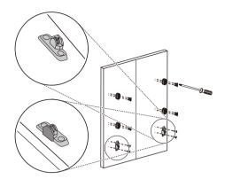
Attach a handle to the front of the cabinet panel before mounting the panel on the dishwasher. Make sure to countersink the screws so the panel slides smoothly.
