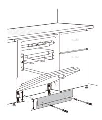
2 Attach a custom toe kick. If needed, use a saw to cut a notch in the top of the custom toe kick to provide clearance for the cabinet panel when opening the door.
