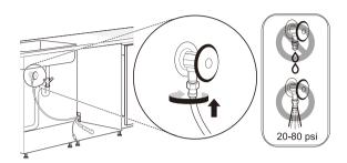
Tighten the connection using a square drive wrench to avoid putting stress on the water tap.
