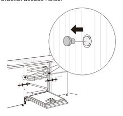
2 Drive a wood screw through the mounting bracket and into the cabinet frame.
