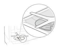
With the lower rack removed, place a level on the inside wall of the tub to check that the dishwasher is level from side to side.
