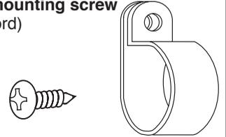
**One power cord clamp bushing** - Actual Size (for the cord hole in a metal upper cabinet)
