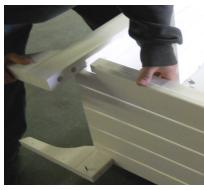
Place top shelf onto top aluminum shelf supports on front and side panels while lightly separating back legs just enough to fit shelf into pocket in legs (Left Picture). Secure using (15) 3/4" Pan Head Screws through aluminum into shelf slats while holding legs tightly to the shelf. (Right Picture)
