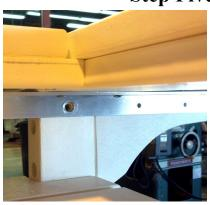
Stand up base assembly. Align long aluminum support on bar top with insert nuts on front legs of base assembly (Left Picture). Secure long aluminum with (2) 3/4" Phillip Pan Head Screws into predrilled holes (Right Picture). Then secure long and short aluminum supports using (12) 3/4" Pan Head Screws.
