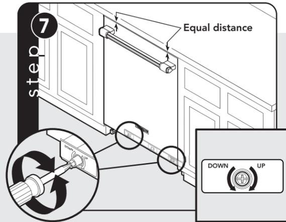
Place a level on handle, then adjust to appropriate height. Left and right adjust side to side and center adjusts front to back.
