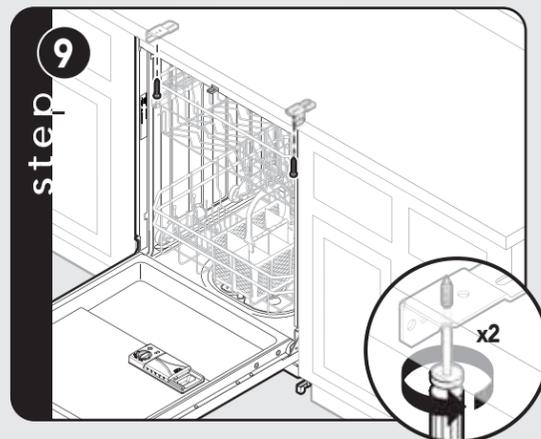
Attach screws through bracket into cabinets.
