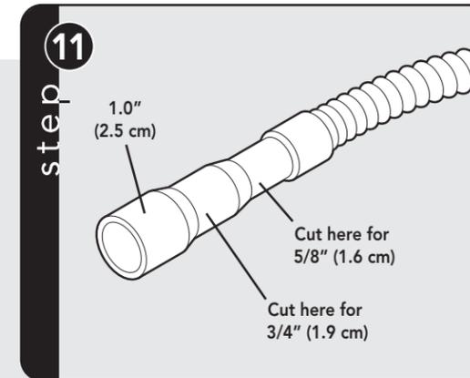
Identify discharge connection size; cut line to correct size and connect. Clamp if necessary.
