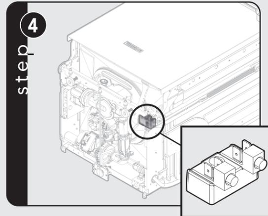
Remove factory installed power cable from terminal block.
