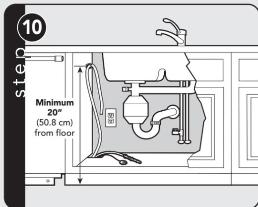
Install High Loop Clip, which is provided, a minimum of 20" (50.8 cm) from the floor. Refer to the Drain section of "General Information" for proper installation requirements.
