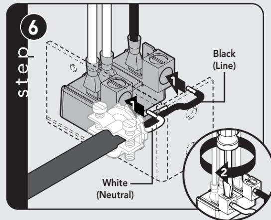
Connect wires to terminal block.
