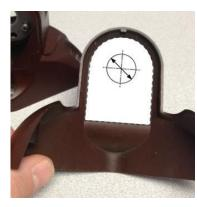
c. Clamp the cover (wings up) to the drilling surface so the part does not shift.
