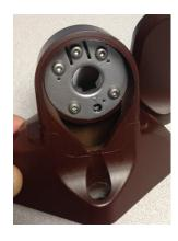
NOTE: If the cover has to be removed, there is a pry slot (on the cover) for a flat blade screwdriver.
