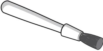
For removing dry pasta residue from the accessories and rollers.
