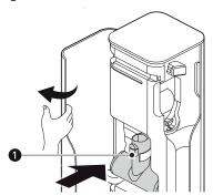
Open the right door and insert the combination tool ②, the crevice tool ③ and the cleaning brush ④ for storage.
