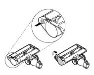
Pull the brush cover forward and pull the main brush out.
