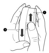
**10** Insert the clean, dry pre-filter and rotate the exhaust filter to the locked position 6 to reassemble it on the product body.
