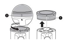
Grip the exhaust filter cover 3 and the exhaust filter **1** using both hands and rotate the exhaust filter cover while pressing the
