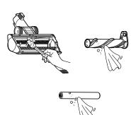
Slide the brush back into the nozzle and rotate the cover back into place. Turn the cover lock clockwise to lock the cover.
