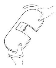
Open the water inlet cap **1** on the middle of the water tank and empty the water tank. Shake the water tank to remove any remaining water.
