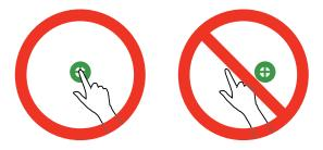
**Note:** Make sure you are not blocking the signal between your finger and the interactive receiver (next to the projector lens).
