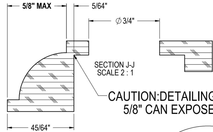
CAUTION:DETAILING EXCEEDING 5/8" CAN EXPOSE LOCK HOLE.
