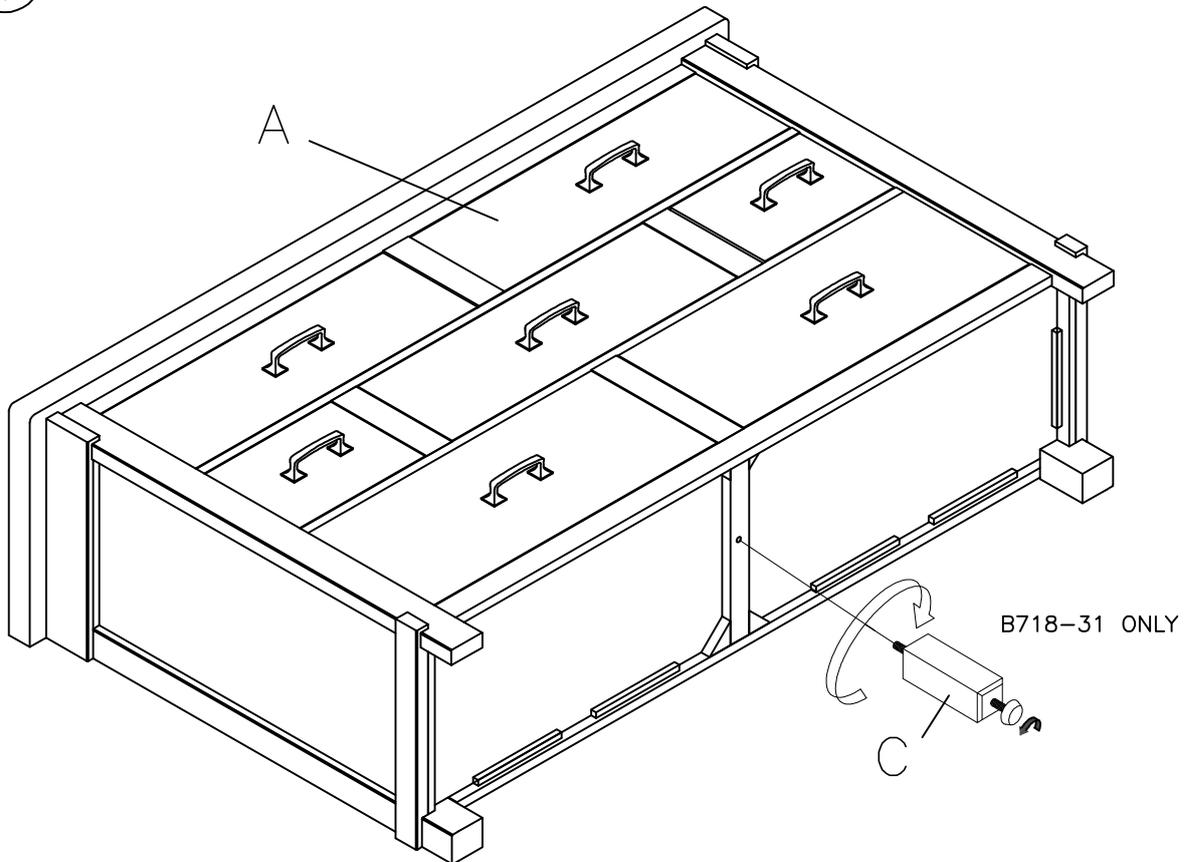
Turn Adjustable Leveler on the bottom of Leg until it contacts the floor.
