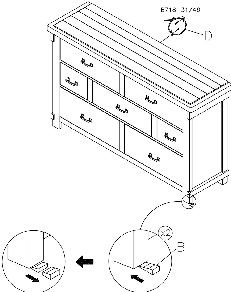
NOTE: IF THE UNIT IS PLACED ON AN UNLEVEL SURFACE, PLACE A LEVELER UNDERNEATH ONE FOOT UNTIL THE UNIT IS LEVEL. BREAK OFF ANY PROTRUDING SEGMENTS.
