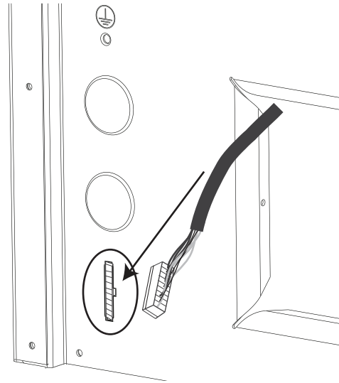
Figure 6: Pigtail Remote Connection
