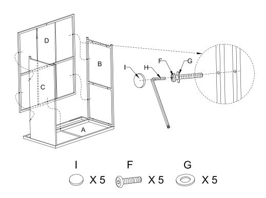
**Step 3.** Attach one shelf (E) to front panel (D), left side panel (B) and right side panel (C) using bolts (F), washers (G), allen key(H) and then cover the bolts with screw caps (I).
