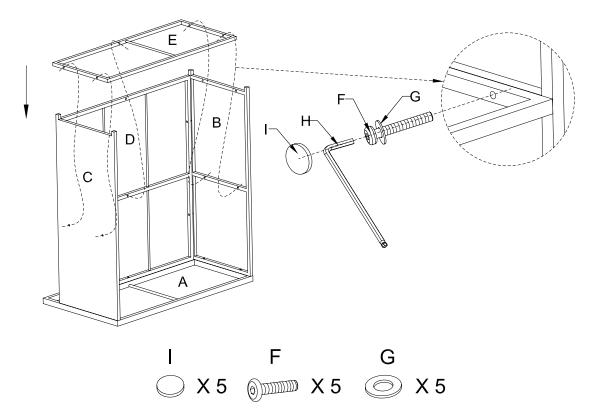
**Step 4.** Attach the other shelf (E) to front panel (D), left side panel (B) and right side panel (C), using bolts (F), washers (G), allen key(H) and then cover the bolts with screw caps (I).
