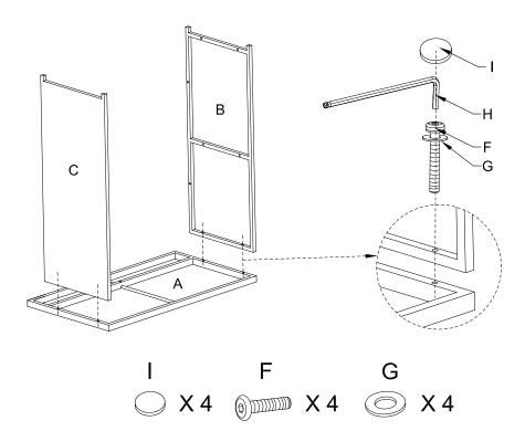
**Step 2.** Attach front panel (D) to top panel(A), left side panel(B) and right side panel (C) using bolts (F), washers (G), allen key(H) and then cover the bolts with screw caps (I).
