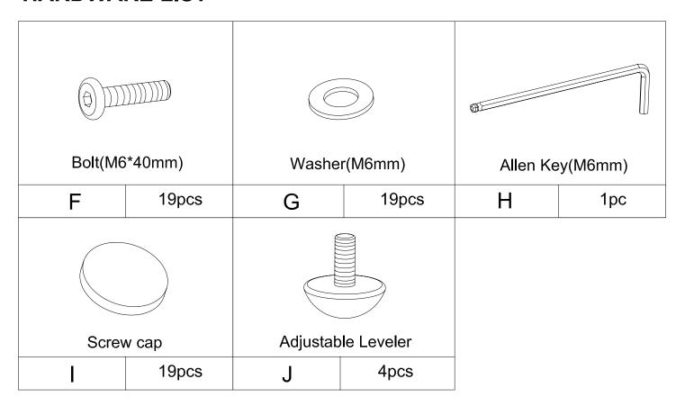
**Step 1.** Lay top panel (A) down on a flat surface with underside facing up.Attach the left side panel(B) and right side panel (C) to top panel (A) using bolts (F),washers (G),allen key(H) and then cover the bolts with screw caps (I).
