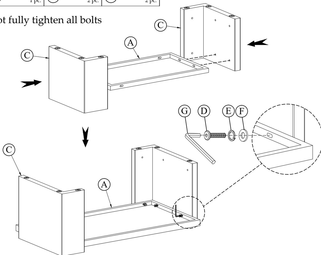
**Step 2 :** Using the Allen key to tighten all bolts.
