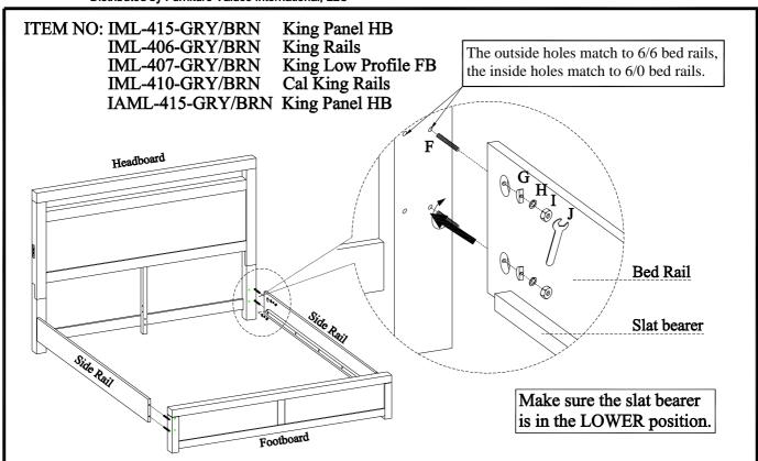
STEP 5: Screw the bolts(F) into HB & FB. Align the bolts with the holes in the end of side rails and attach the side rails to HB & FB using half moon washers(G),lock washers(H) and nuts (I). Then use a hex wrench to tighten all the nuts.
