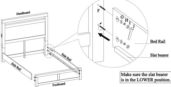
STEP 5: Screw the bolts(F) into HB & FB. Align the bolts with the holes in the end of side rails and attach the side rails to HB & FB using half moon washers(G),lock washers(H) and nuts (I). Then use a hex wrench to tighten all the nuts.
