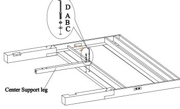
STEP 2: Attach the center support leg to headboard by using 2 bolts(A), lock washers(B) and flat washers(C).
