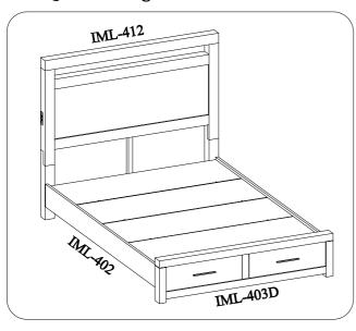
All Beds need to be set up in the exact final location so that after full assembly it will not need to be moved. Moving the bed will cause the support legs to move out of perpendicular (90 degree), weaken the support system, and may allow the bed to collapse.
