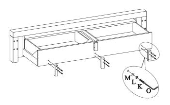
STEP 4: Attach support legs (for pedestal) to footboard.
