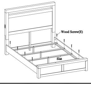
STEP 7: Arrange the slats on the slat bearers equally and attach to the slat bearers with wood screws (E).
