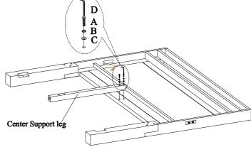
STEP 2: Attach the center support leg to headboard by using 2 bolts(A), lock washers(B) and flat washers(C).
