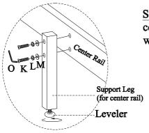
STEP 8: Attach 2 support legs (for center rail) to the center rail using 4 bolts( K), lock washers(L) and flat washers(M). Use an Allen Wrench to tighten all the bolts.
