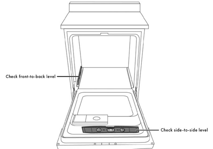
2. Level the dishwasher by adjusting the three leveling legs individually.
