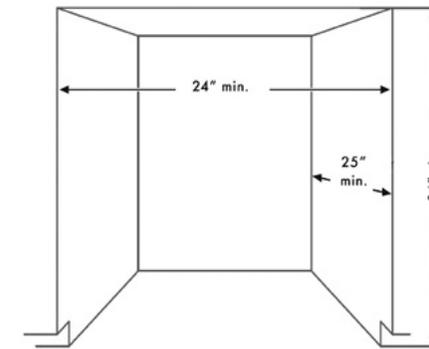
If installing into a corner, allow 2 in. min. clearance between dishwasher and adjacent cabinet, wall, or other appliances. Allow 25.63 in. min. clearance from the front of the dishwasher for opening the door.
