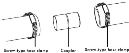
3. Secure the drain hose to the air gap, waste tee, or garbage disposal with a screw-type clamp, using the appropriate method below. See "Drain Preparation" on page 6, if you do not know which method to use.
