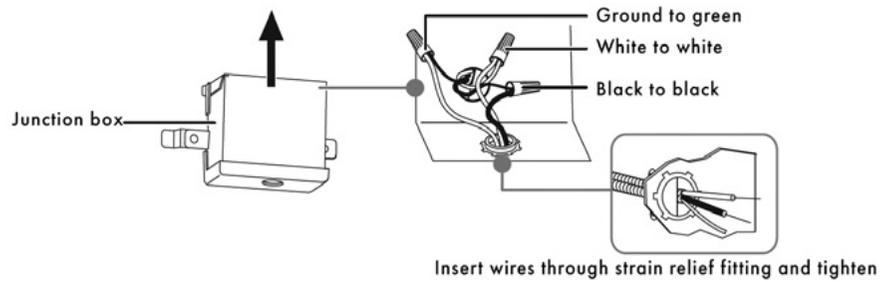
2. Locate the three dishwasher wires, (white, black, and green) with stripped ends, then insert the dishwasher wires through the small hole in the junction box.
