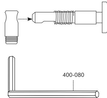
**B.** Install the cross dowels into both ends of the spanner post as shown. Gently tighten the set screw in place with the hex key. (Adjust set screw to move dowel fastener in and out as needed.)
