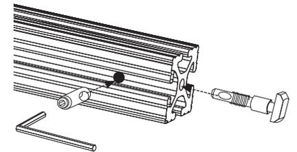
**C.** Slide the spanner post into the front two riser posts.
