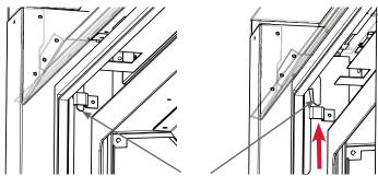
Hooks on mesh barrier frame
