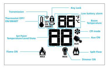
Figure 2: Transmitter LCD Display
