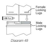
5. Assemble the desired combination of pipe and elbows to the appliance adaptor and twist-lock for a solid connection.
