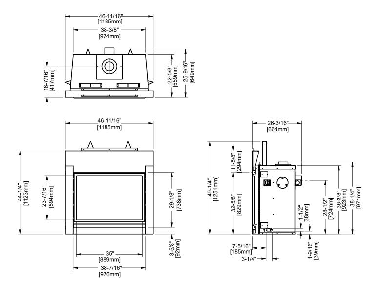
Note: Gas connection is from the right hand side of the appliance & electrical connection on left hand side of the appliance. A metal receptacle box is supplied/installed with the appliance to make all 120 volt electrical connections.
