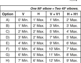
With these options, maximum total pipe length is 30 feet with minimum of 6 feet total vertical and maximum 8 feet total horizontal. Please note minimum 1 foot between 90° elbows is
