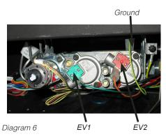
11. Remove the 14 screws securing the valve tray assembly in place (Diagram and then lift the entire assembly out Also remove the valve gasket.
