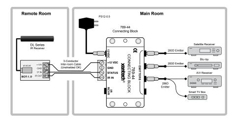
a more distant location, you may splice in 2-conductor wire, in the wire gauges mentioned before, as needed.
