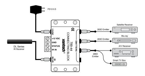
The IR receiver is in close proximity to the audio/video equipment, no wiring extension should be required so long as the connecting block is within reach of the 7-foot cable. The 3.5mm stereo type mini plug is connected to the "IR RCVR" jack on the Xantech Connecting Block.
