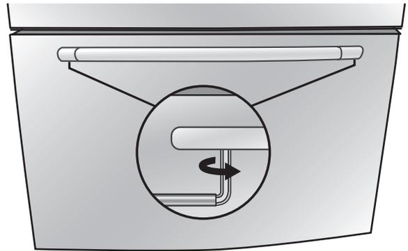
4. Using a left-to-right motion, tighten the setscrew a quarter turn at a time just until it begins to contact the shoulder screw. Do not fully tighten.
