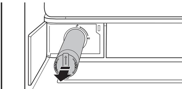
4. Remove the water filter cap from the water filter.
