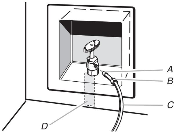
A. Sleeve B. Nut C. Copper tubing (to refrigerator)
