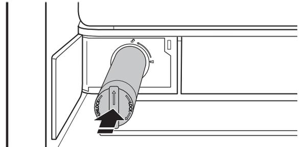
7. Twist the water filter and turn 90° clockwise until it locks into place and that arrows are aligned.
