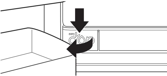
2. Twist the water filter and turn 90° counterclockwise to unlock.
