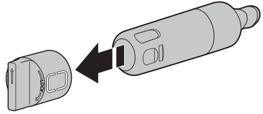
5. Install the water filter cap onto the new filter. Be sure to align the arrows so the grooves in filter align with ribs in filter cap.
