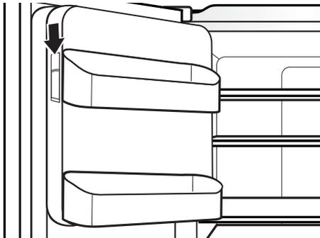
2. Turn on the ice maker by moving the switch to the On (I) position.
