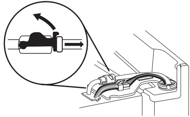
3. Disconnect the wiring plug located on top of the door hinge.
