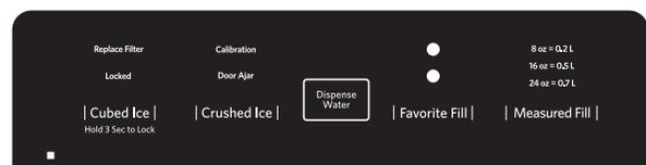
**IMPORTANT:** The display screen on the dispenser control panel will turn off automatically and enter “sleep” mode when the control buttons and dispenser paddles have not been used for 2 minutes or more. Touch any control button to reactivate the display screen.
