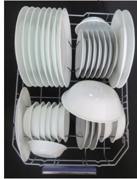
Bottom rack load pattern for 10 place settings
