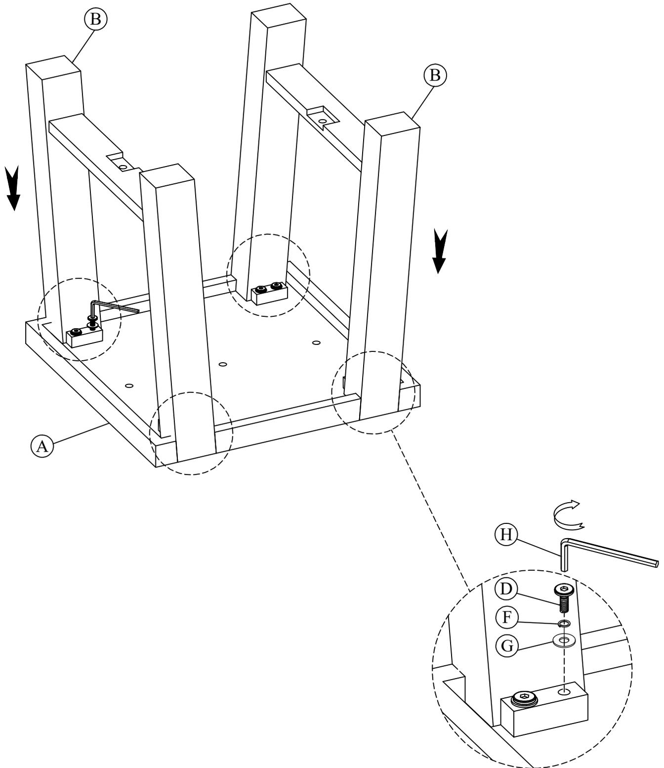
**Step 3 : Using the Allen key to tighten all bolts**
