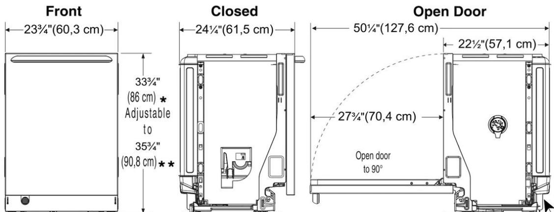
\*\* Height only adjustable to 35 3/4" (90,8 cm) max when installed in 35 3/4" (90,8 cm) max standard cabinetry cutout. to 35 3/4"
