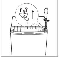
**4.** Unscrew bottom hinge. Remove adjustable feet from both sides.
