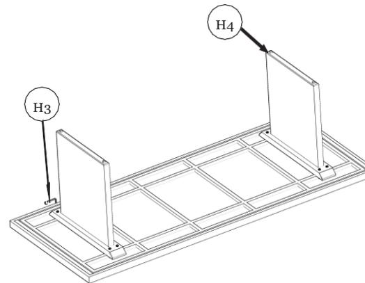
USE THE ALLEN KEY TO SCREW THE ALLEN BOLT FROM THE BOTTOM OF THE TABLE TOP
