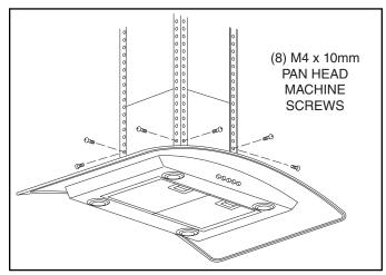
Assemble (4) angle brackets to the hood using (8) M4 x 10mm pan head machine screws (2 for each angle bracket).
