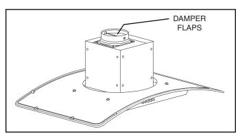
Remove the damper flaps from the damper / duct connector and discard flaps.
