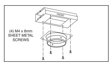
Attach non-duct collar to non-duct plenum using (4) M4 x 8mm sheet metal screws.
