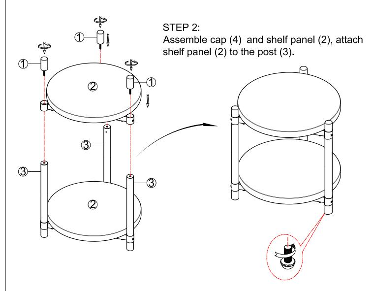
Adjust leveler if needed to level table on uneven floor.
