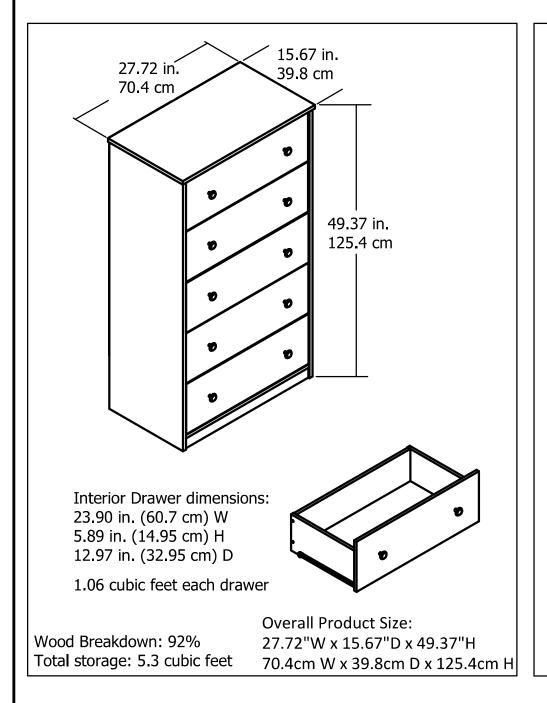
25 lbs 11.3 kg (each drawer) 50 lbs 22.7 kg Maximum Weight Capacities Unit Weight: 89 lbs. (40.4 kg)
