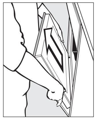
■ Holding the door securely at both sides, lift it straight upwards.
