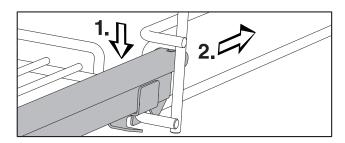
■ Insert the FlexiClips with wire rack onto the level (1.) and slide it along the struts of the level (2.) until it clicks into place.
