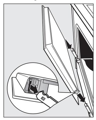
■ Hold both sides of the door securely and carefully fit it onto the brackets of the hinges.
