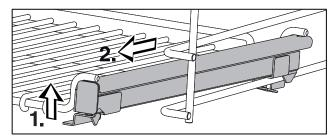
■ Using both hands lift the front of the FlexiClips with wire rack on both sides (1.) and pull it out of the level (2.).
