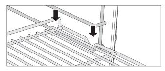
Always place the wire oven rack on the runner with the notch facing down.
