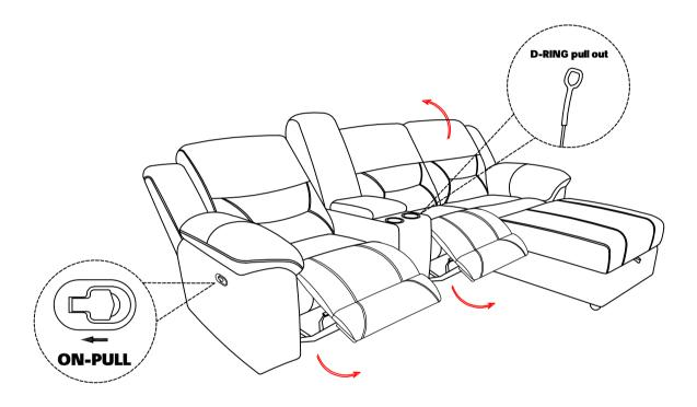
Open the Footrest by pulling out the Switch.
