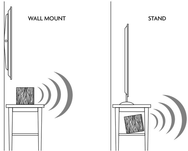
NOTE: When the center channel is positioned below ear level, it should be angled upward as seen in the diagram above.
