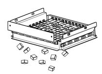
The bin level sensor is located in the ice bin, it senses when the ice supply is low or full and starts or stops the ice making process accordingly.
