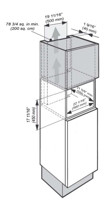
Lower gap adjustment detail when solo installed.
