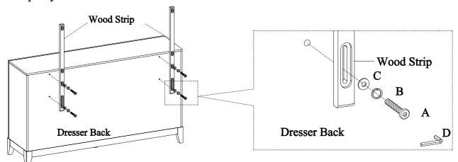
STEP 2: Attach the wood strips to the mirror by using 4 bolts(A), lock washers(B), and flat washers(C). Tighten all bolts on dresser and mirror with Allen wrench.
