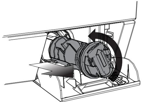
Inspect for O-ring before reinserting pump filter
