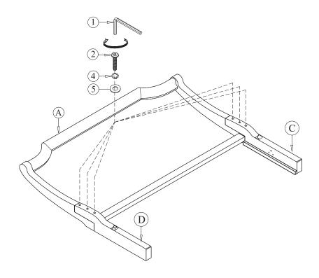
STEP 2 Assemble the headboard cross bar (E) to headboard legs (C & D) by using Allen Key (1) with hardware 3, 4, and 5. \*TIGHTEN ALL THE BOLTS BY USING ALLEN KEY (1)
