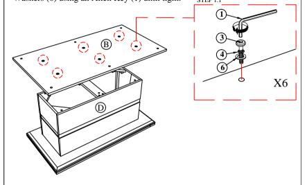
**STEP 3 :** Place the Table Top (A) upside down on a soft surface, then turn the Table Leg (D) upside down and place it under the Table Top (A) as shown below. fasten the screw JCBC Bolt (2) together with Spring Washer (4) & Flat Washer (6). Fasten until tight.
