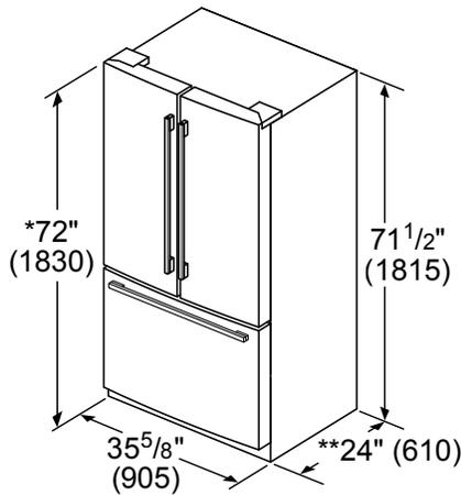
\* Add  $\frac{5}{8}$ " (17) with front leveling feet fully extended
