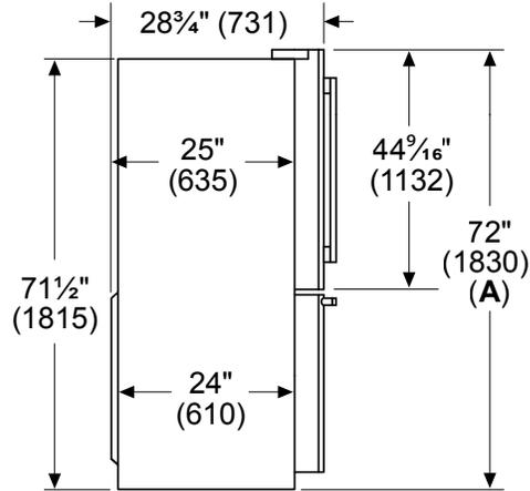
A: Add  $\frac{5}{8}$ " (17) with front leveling feet fully extended
