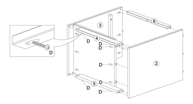
Secure front cross beam (4,5,6) to panels (2,3) using screw (D)
