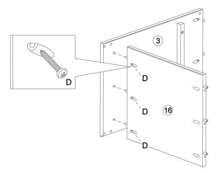
Secure base (16) to panels (3) using screw (D)
