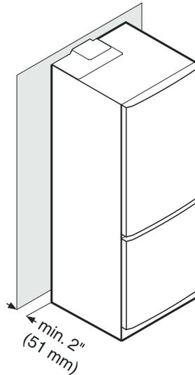
Clearance on the back must be 2 inch (51 mm).
