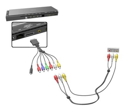
If you are using the One Connect's AV2 input connectors, use the included AV connection adapter to connect the device's audio and video output to the TV.
