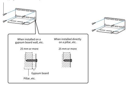
The distance between the mounting brackets should be between 675 mm to 920 mm.
