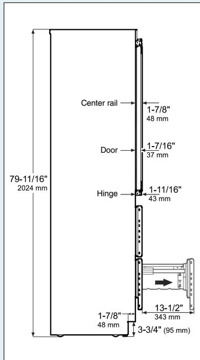
Height can be increased by 1-1/2" (40 mm) by turning the levelling feet at the front and the height adjustable roller units at the appliance rear.
