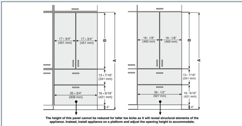
The height of this panel cannot be reduced for taller toe kicks as it will reveal structural elements of the appliance. Instead, install appliance on a platform and adjust the opening height to accommodate.
