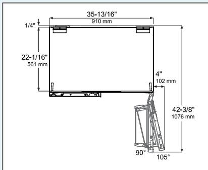
Allow door swing clearance at locations next to a wall. The refrigerator door must open to a minimum of 90° to allow the crispers to open and the shelves to be removed.
