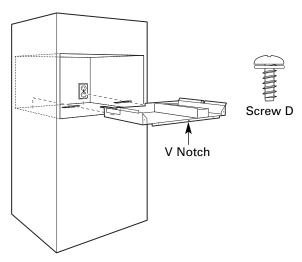
B Slide the two Base Support Brackets from the rear into the slots in the Base Pan. The tongues of the Base Support Brackets should protrude into the base, be centered in the slot, and be into the slot as far as they will go. Mark and drill four 3/32" diameter holes. Mount the Base Support Brackets using four Screws (D). Both Base Support Bracket tongues should now be centered in the slotted holes in the base and be into the base as far as they can go.
