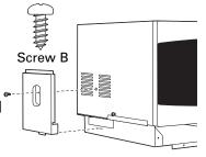
the side bracket with the dimple in the oven. Carefully drive one screw (B) through the Side Bracket into the side of the oven, using a screwdriver or power drill. Be sure the Side Bracket is tight against the side of the oven.
