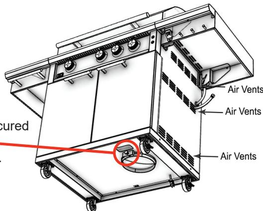
**NOTE:** LP Tank is secured in the cart by a bolt which locks it in place.
