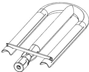
The performance series stainless U-Style XLT burner is used in this XO gas grill. This new burner has even heat distribution that enables rapid heating throughout the cooking area.
