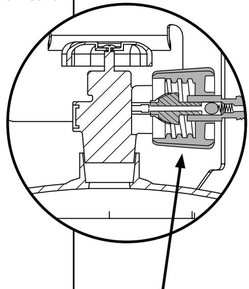
Hand tighten to ensure proper seal for correct gas flow.
