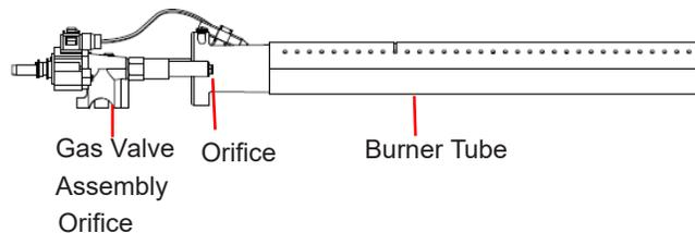
Please Note that the air mixture for LP gas and NG is different. Your gas grill will come preset for your gas type. If you find that you are not getting the best flame you can adjust the air shutter and the O2 mix with gas will change the flame. The flame coming from your burner is extremely important. If the flame is not correct you will be able to adjust the flame as described in the section below.
