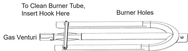
For safe operation ensure the Gas Valve Assembly Orifice is inside the Burner Tube before using your grill. (See figure above). If the Orifice is not inside the Burner Tube, lighting the Burner may cause explosion and/or fire resulting in serious bodily injury and/or property damage.
