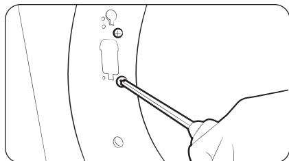
8. Re-insert the two screws that held the lever holder into the same screw holes, and then tighten.
