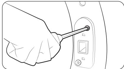
12. Push the lever holder into the cut out on the other side of the door opening. Insert screws, and then tighten as shown.
