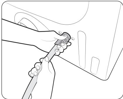
1. Connect the angled end of the water hose to the filling valve at the bottom rear of the dryer. Turn the coupling by hand until it is tight.
