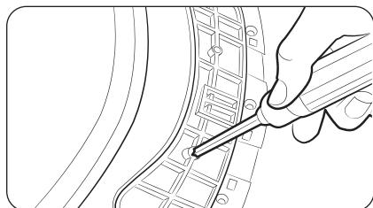
9. Remove the single screw from the back of the door hinge.
