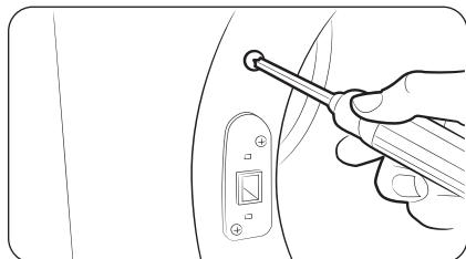
6. Remove the two screws above and below the lever holder on the opposite side of the door opening.
