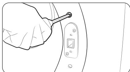
13. Re-attach the remaining screws to the remaining holes above and below the lever holder, and then tighten.
