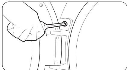
11. Place the door on the other side, and then reattach it to the dryer.
