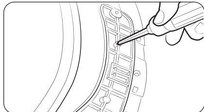
10. Insert the screw you just removed into the other screw hole on the back of the door hinge, and then tighten.
