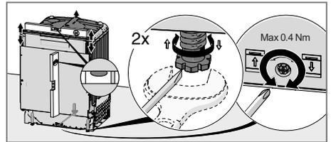
4. Verify there is an air gap of at least 0.1" (3 mm) between the underside of the countertop and the top edge of the dishwasher.
