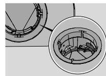
Check that the colored stop on the right in the bottom drain is in place.
