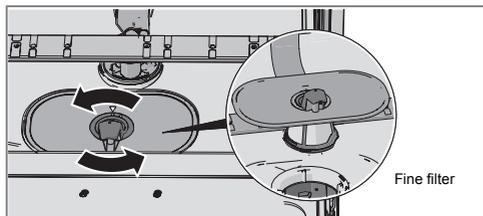
1. Turn the locking ring counterclockwise and lift the fine filter straight up.
