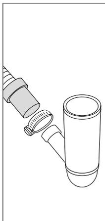
The drain hose can also be connected to a connection nipple on the sink unit's water trap. The connection nipple must have an internal diameter of at least 0.6" (14 mm).
