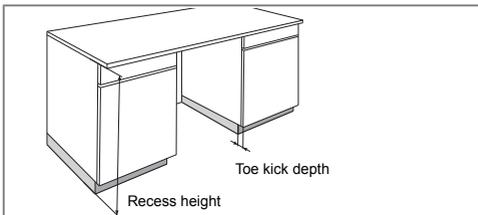
Use a sharp knife to score the front and the back of the toe kick at the desired height. Now carefully separate the two pieces to form a toe kick of the right height.
